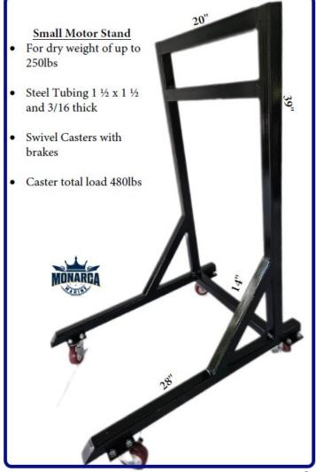
The small motor stand is great for your smaller horse power engines, but still built sturdy and sealed to avoid water intrusion and corrosion.
