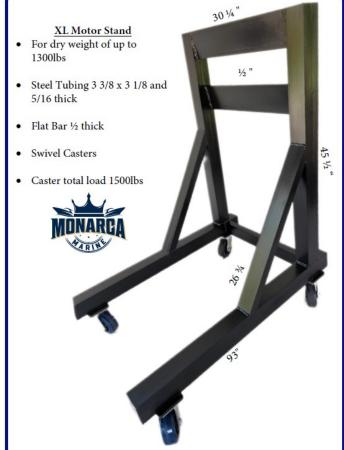
The XL stand is perfect for your heigh performance engines, strong enough to hold 1300lbs, sealed to avoid water intrusion and corrosion.
